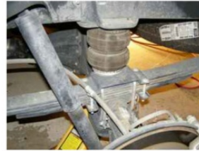
Aftermarket/Secondary Air Suspension (Air Bag Supplements the Primary Leaf Spring Assembly)
