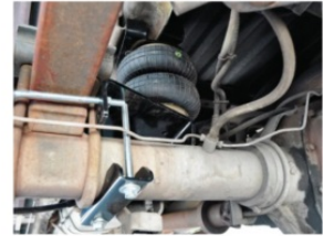
Aftermarket/Secondary Air Suspension (Air Bag Supplements the Primary Leaf Spring Assembly)
