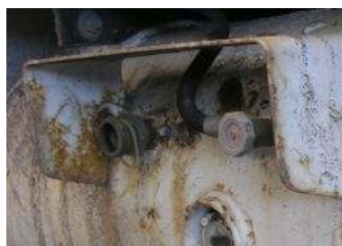
Fuel tank filler cap missing
